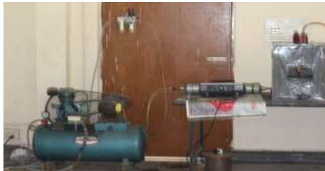
Fig 4.10: Assembled abrasive hot air jet machine setup
